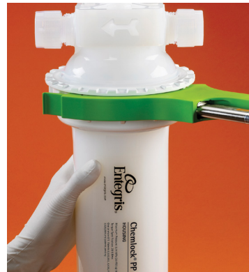
4. Tighten locking ring to easily seat double o-rings. Use a Chemlock integrated housing wrench to ensure proper tightening.
